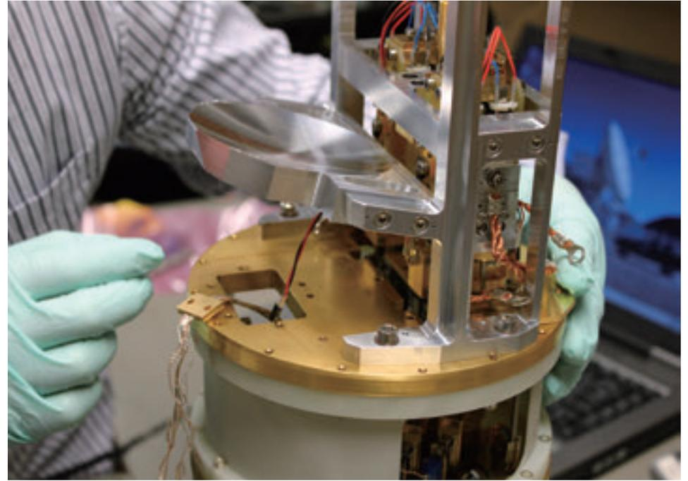
Left: Band 9 receiver cartridges delivered by NOVA, the Netherlands. Credit: ESO/NOVA
