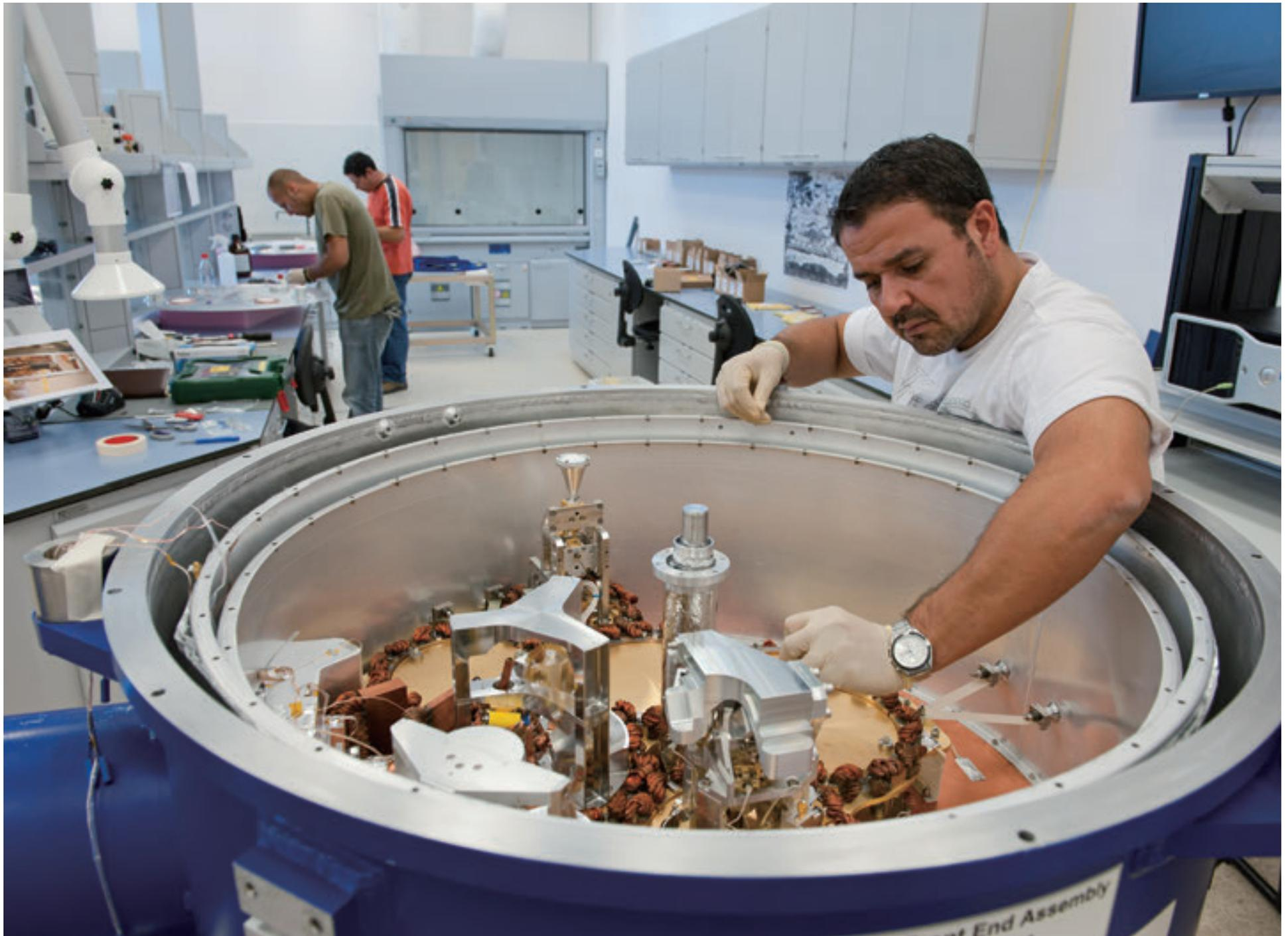
A cryogenics and vacuum technician assembling an ALMA cryostat. Credit: ESO/M. Alexander
