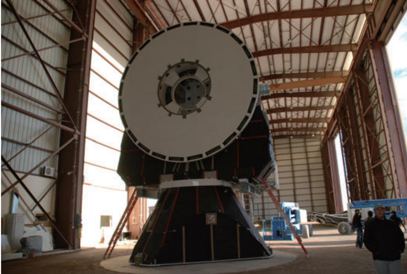
The assembly of a North American antenna in the Site Erection Facility building at the OSF. Credit: NRAO/AUI
