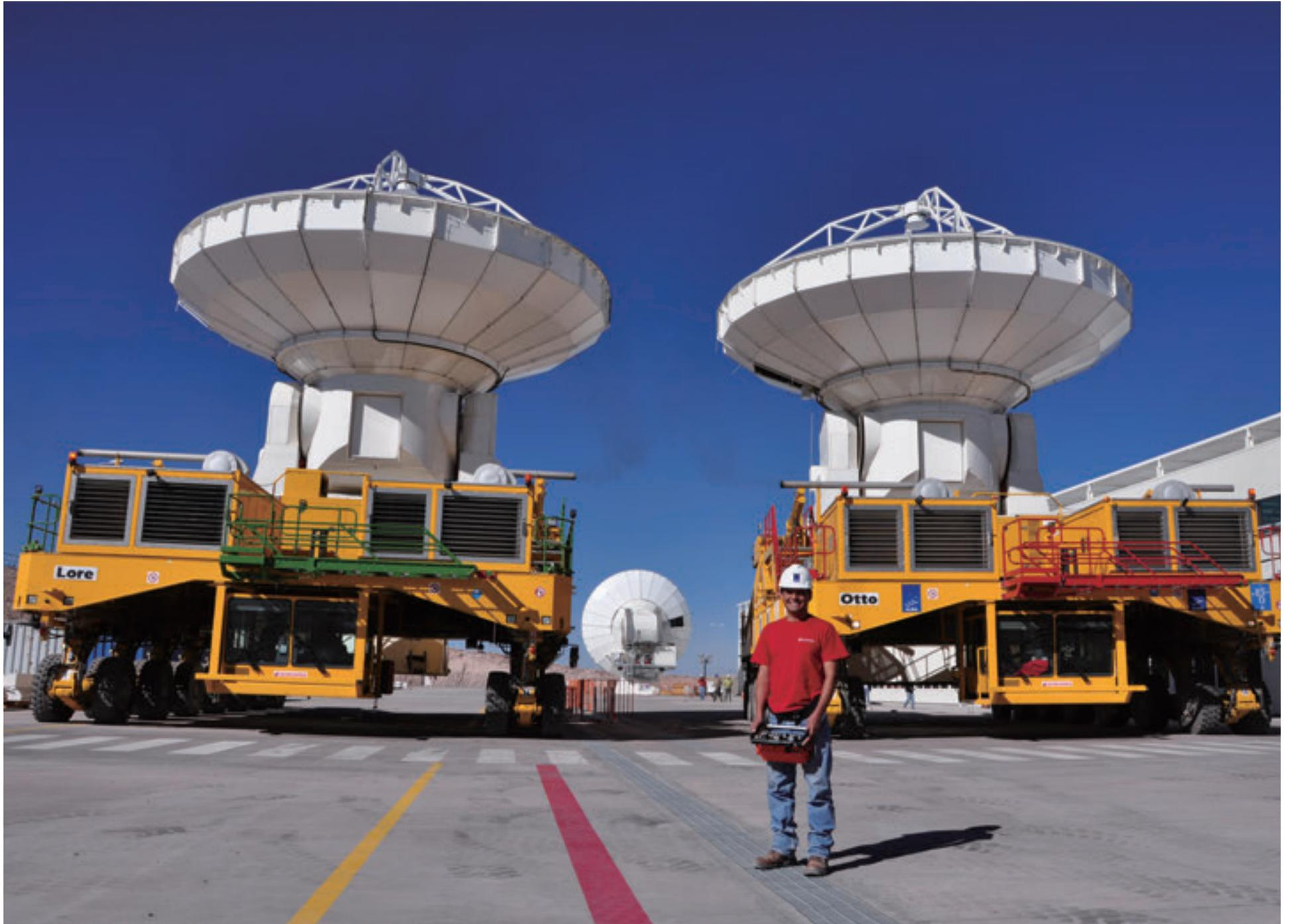
Simultaneous transfer of two antennas with Otto and Lore, the two ALMA transporters. Credit: ALMA (ESO/NAOJ/NRAO)
