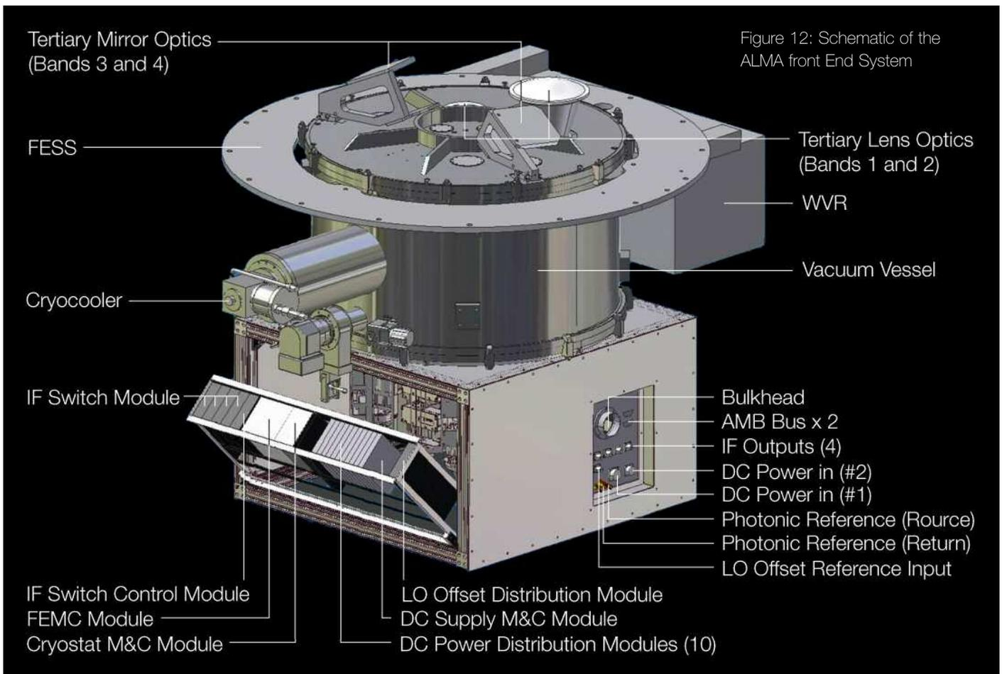
Figure 12: Schematic of the ALMA front End System
