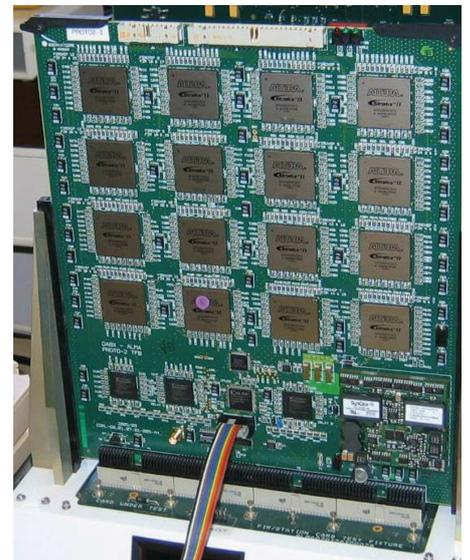
Figure 18: Tunable Filter Board Card Developed by the University of Bordeaux
