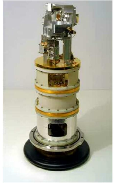
Figure 14: Band 9 Receiver Cartridge assembled by NOVA
