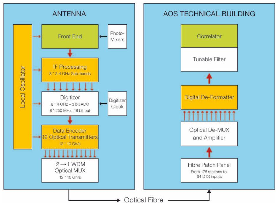
Figure 15: Schematic of ALMA Signal Processing and Data Transfer from the Front End to the Correlator. Parts to be provided by ESO are shaded in yellow.
